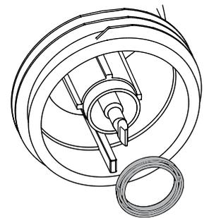
7. The units may only be used with a functional valve. If paints rises in the ventilating hose (Fig. 1, item 19) do not operate the unit further! Dismantle and clean the ventilating hose, valve and diaphragm and replace the diaphragm if necessary.
